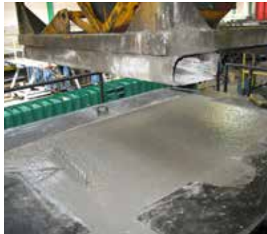
Complicated steel cage structures are eliminated from BarChip concrete elements.
